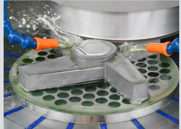
Water cooled closed-circuit system and magnetic chuck to fix the blades
