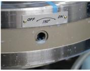
The APB401 uses a keyway to activate the magnet that holds the plate firmly to the spindle base.
