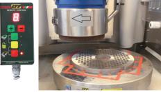
The APB401E uses an adjustable electromagnet to hold the plate firmly to the spindle base.
