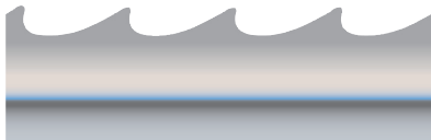
Style #325P - 3 teeth/in. Gauge .025 Width 3/4"
